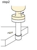
Spindle runs about 500 rpm. Move spindle close to measuring surface.
